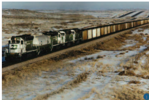
Burlington Northern dual-fuel natural gas tandem with LNG tender in service hauling coal. Has range of 800 miles between refueling stops.
