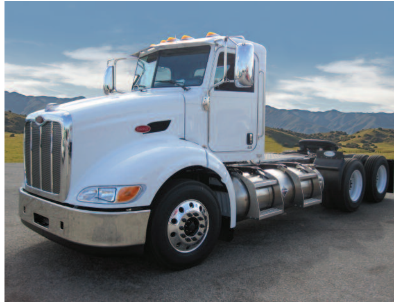
Peterbilt truck consumes five percent diesel and 95 percent LNG with no loss of torque or power. (Courtesy Peterbilt)
