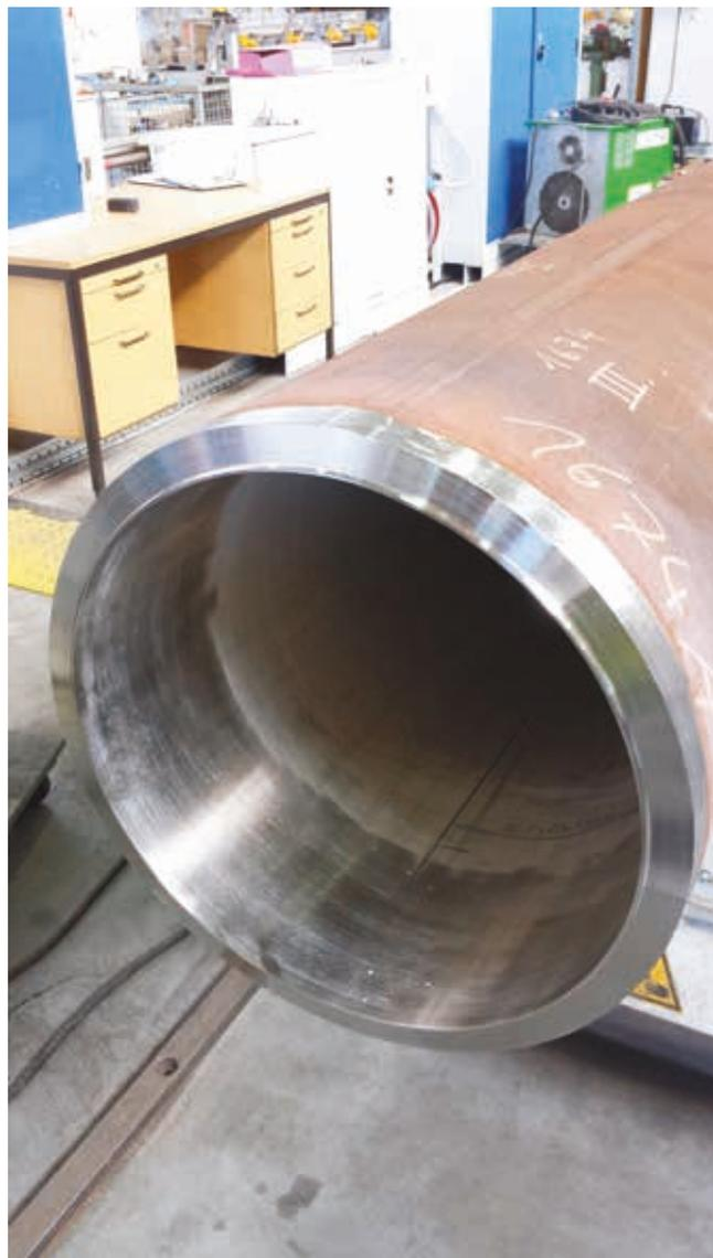
**Figure 4. Internal view of CRA lined pipe. The machined weld overlay at the pipe end and the weld preparation show the thin lip of CRA material that needs to be carefully aligned with the next pipe.**
