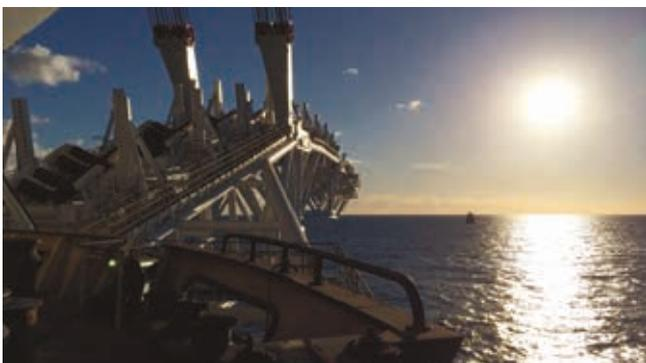
Figure 2. Allseas pipelay vessel *Audacia* with elevated stinger prior to commencing pipelay.
