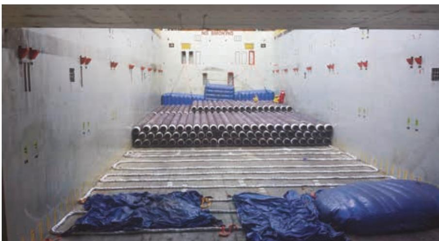
**Figure 7. Stowage of suitable preserved CRA lined joints within the pipe transportation vessel hold.**
