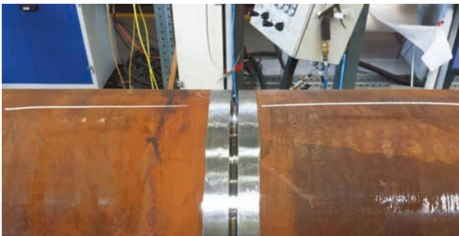
**Figure 6. Precise alignment of pipe ends is required before welding operations can begin.**
