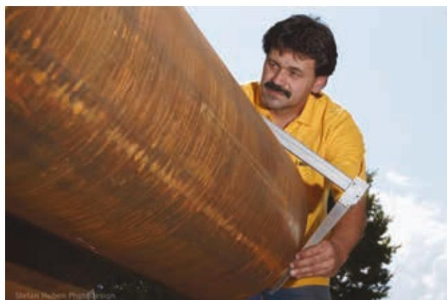
**Figure 5. Dimensional control of CRA clad and lined pipes is crucial to allow efficient welding operations.**
